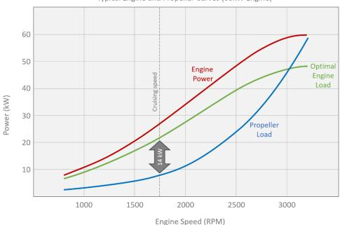
Typical Engine and Propeller Curves (60kW Engine)
